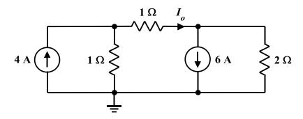
a. How many equations are necessary to analyze this circuit by the nodal analysis method?
